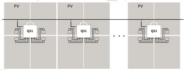
In the 2X2 configuration above, DC extension cables are not required.
