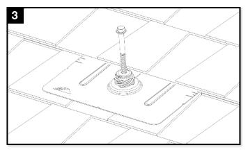
Line up pilot hole with flashing hole and insert lag bolt with bonded washer through flashing. Tighten lag bolt until fully seated.
