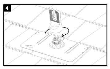
Place Cap onto flashing in desired orientation for E/W or N/S rails and rotate 180 degrees. FlashFoot 2 is now installed and ready for IronRidge XR Rails.
