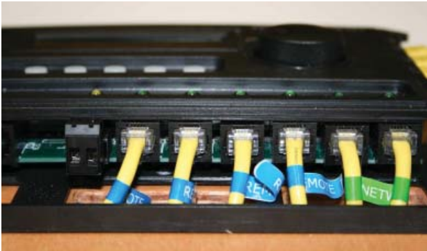
Figure 2-6, Concealed Mounted Remote/Network Cables
