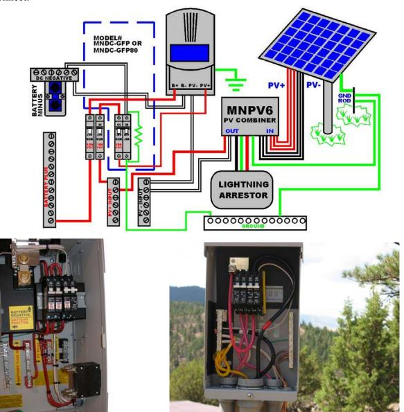
Cut out spaces to allow for the breaker assembly. Make sure the yellow snaps are totally snapped onto the din rail. Torque to 20 inch pounds. Re-torque one hour later. Sometimes wires cold flow and loosen up upon initial clamping.
