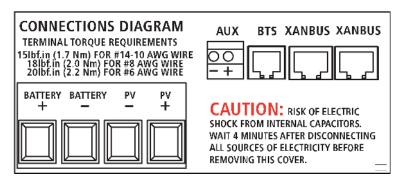
Figure 2-9 DC Connection Terminals
