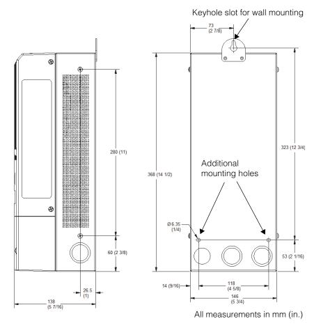
Figure 2-3 Dimensions and Knockout Locations
