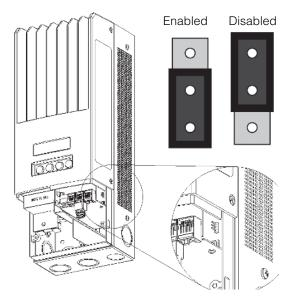
Figure 2-7 PV Negative Ground Jumper Location
