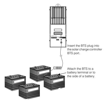
Figure 2-16 Installing the BTS
