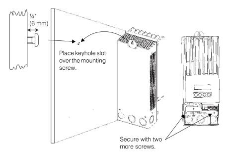
Figure 2-5 Mounting the Conext MPPT Solar Charge Controller
