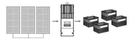
Figure 1-3 PV Charge Controller
