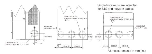
Figure 2-4 Knockout Dimensions
