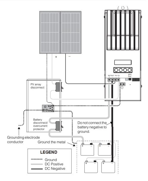
Figure 2-10 Charge Controller Power Wiring
