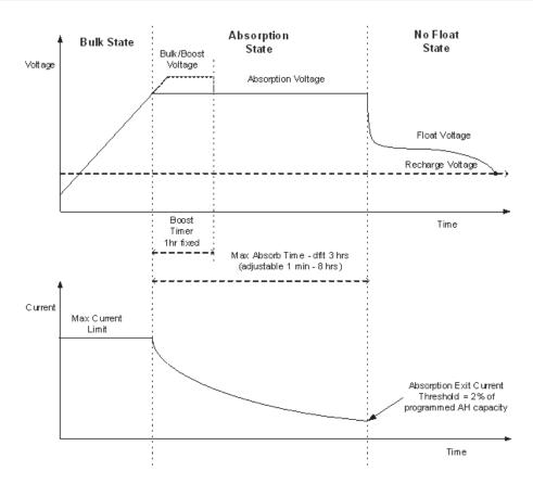
Figure 1-5 Two-stage Battery Charging Cycle
