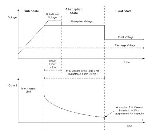
Figure 1-4 Three-stage Battery Charging Cycle<sup>a</sup>
