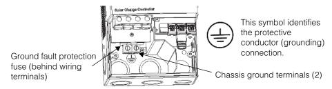
Figure 2-6 Charge Controller Safety Ground Connector
