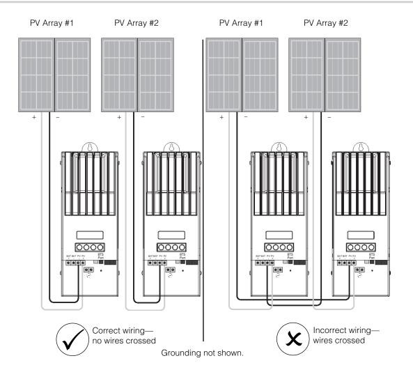
Figure 2-11 Multiple Charge Controller Array Wiring
