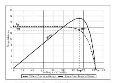
Figure 1-2 Maximum Power Point Curve
