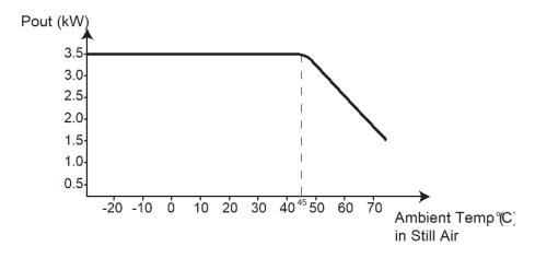
Figure A-1 Output Power vs. Ambient Temperature
