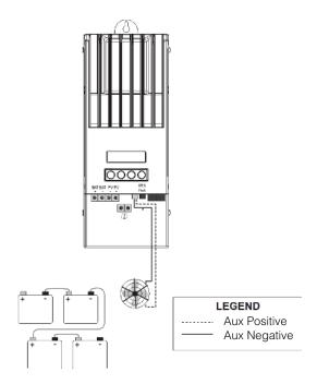
Figure 2-12 Auxiliary Output Vent Fan Application
