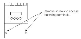
Figure 2-2 Removing the Wiring Compartment Cover
