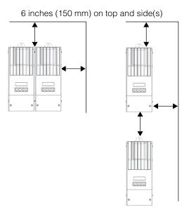
Figure 2-1 Minimum Clearance Requirements
