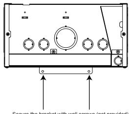
Secure the bracket with wall screws (not provided)
