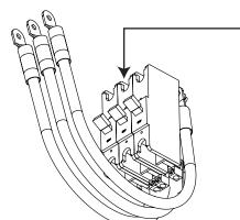
Re-attach the assembly to the DC breaker mounting rail using the front mounting screws (two per breaker)
