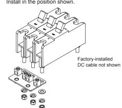
6 Connect the positive (red) DC cable provided with the Connection Kit to the stud terminal on the back of the additional breaker(s)
