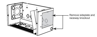
Either sideplate can be removed depending on the location of the adjacent PDP and Conext XW+. If the Conduit Box is located between two XW+ units, then remove both sideplates and knockouts.
