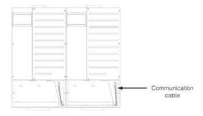
**Note:** In a dual-inverter system, install an AC Sync Cable from INV1 to INV2. In a triple-inverter system, daisy-chain an AC Sync Cable from INV1 to INV2 and from INV2 to INV3.
