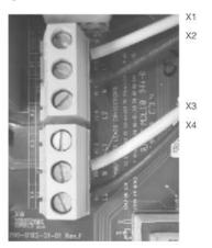
Secondary transformer wire X1, X2, X3, and X4 locations BEFORE reconfiguration
