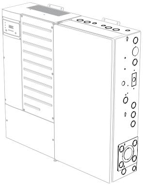
Remove your choice of knockouts from the XW Pro chassis, Conduit Box, and/or Power Distribution Panel (PDP). Verify that no debris remains inside the chassis. Insert appropriately-sized conduit bushings into each conduit hole.
