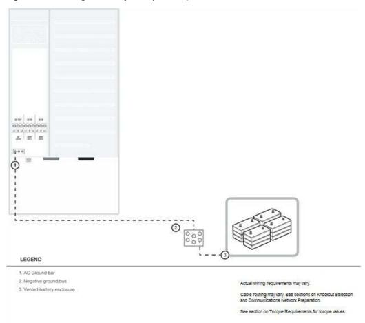
Figure 57 DC Connections to a Single Inverter (No PDP)
