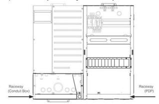
Before making AC and DC connections, route communication cables (including Battery Temperature Sensor) through the raceways. For easier identification, use a different color for each communications cable, or cable tags.
