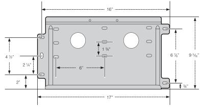
**Note:** If the wall does not have 16-inch on-center studs, you will need to provide adequate support for the Mounting Plates. For example, a sheet of fire-rated plywood<sup>2</sup> can be attached to the wall, and the Mounting Plates can then be attached to plywood.
