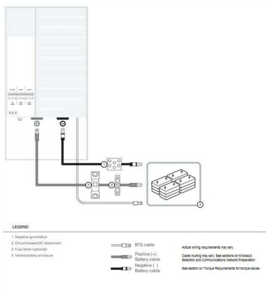
Figure 58 Grounding the AC System (No PDP)
