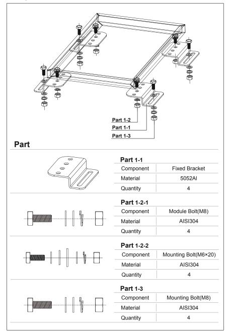
Attached the PV module to the mounting foot using M8 screw/bolt supplied in the pack. Be carful of the bolt, flat washer, spring wash and nut sequences. Find suitable holes on the panel frame and fasten the mounting foot on it.
