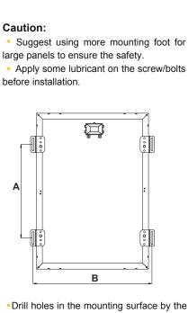
Drill holes in the mounting surface by the length of A and B measured from the panel before installation. Mount the panel together with the holes.
