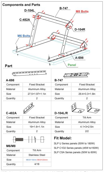
\*(M6) all 4 mounting bolts will be used to install A-698(fixed bracket) to the PV module frame. Place 1 mounting bolt on each of the 4 sides of the PV module frame.
